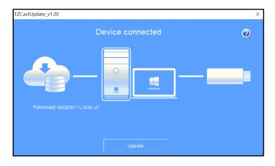
Step7. Now the system is installing the latest firmware. **Please be advised** that DO NOT turn off the power of QuattroPod Transmitter during the process.
