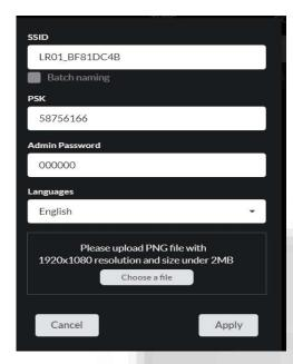
**SSID:** Support renaming and batch renaming by adding the serial numbers.
