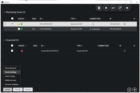
Within this option the user can change the name of the SSID and PSK. The Admin will also be able to introduce a New Admin Password and Change the language. There is also an upload file which allows users to upload the customized wallpaper.
