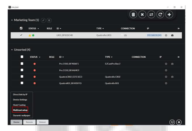
The main purpose of the Multicast is to allow users streaming from one transmitter to the multiple receivers. It is a one-to-many function. The user needs to set a group first. The QuattroPod receiver must be connected to a router. So the Router SSID and the password should be entered.
