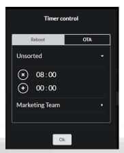
**3.2 OTA:** As for the OTA control. We can set a timer to notify the device to check whether there is newer firmware version. The timer can be set "D" on a daily basis, "W" on a weekly basis, or "M" on a monthly basis.
