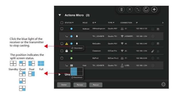
To select the position to split screen, simply move the mouse and it would preview where the transmitter would cast.
