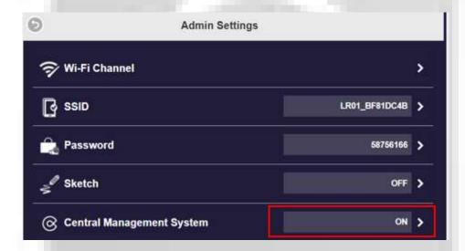
After doing this the administrator user must refresh the CMS dashboard. If the "Central Management System" switch is off the device will be undiscoverable, you can confirm this by checking the status bar in the dashboard, if the status is in red the device is undiscoverable, if the status is in green, the device is discoverable.
