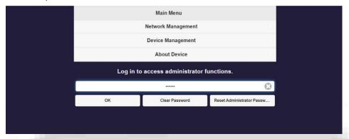
To connect your EZCast Pro device, go to Network Management. Press "Connect to 5gHz Wi-Fi".
