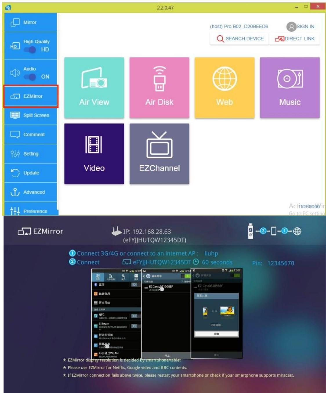
EZMirror is fully compatible with Miracast. You can click the EZMirror button in EZCast app, and the receiver will be switched to Miracast mode.
